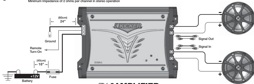
Figure 2 Two Channel Operation (Stereo) Minimum Impedance of 2 ohms per channel in stereo operation
